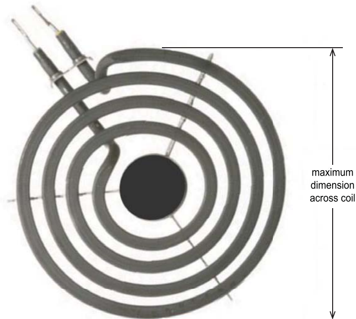
Figure 60A.2 Determination of coil heating element size
