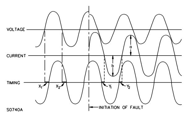
Current = [ (a+b)/2] (rms calibration of instrument element)
