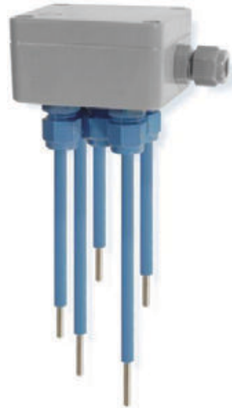
FIG. 3.9d Conductivity switch with five probes can control a filling operation in four stages. (Courtesy of B + B Sensors.)
