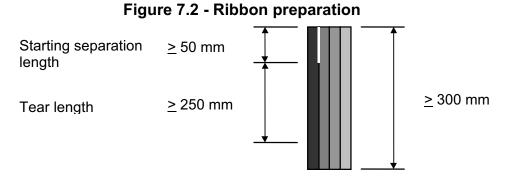
Note: Tear length (Figure 7-2) as shown.
